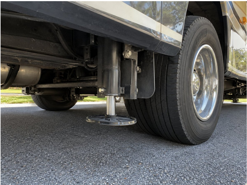
Illustration: Hydraulic jack below its fully stowed position.
