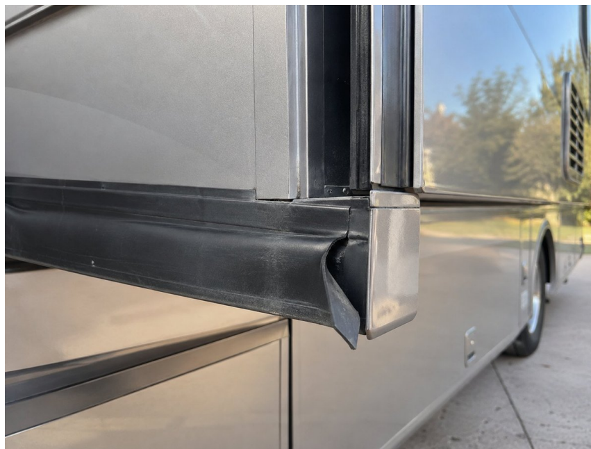
Illustration: Localized tear in the lower slideout sweep.
