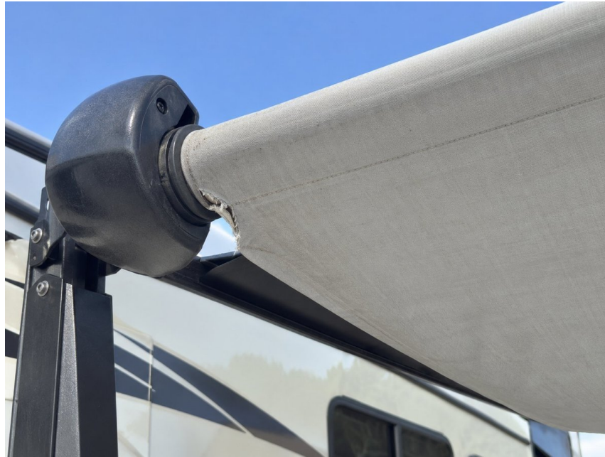
Illustration: Localized tear near the patio awning roller edge.
