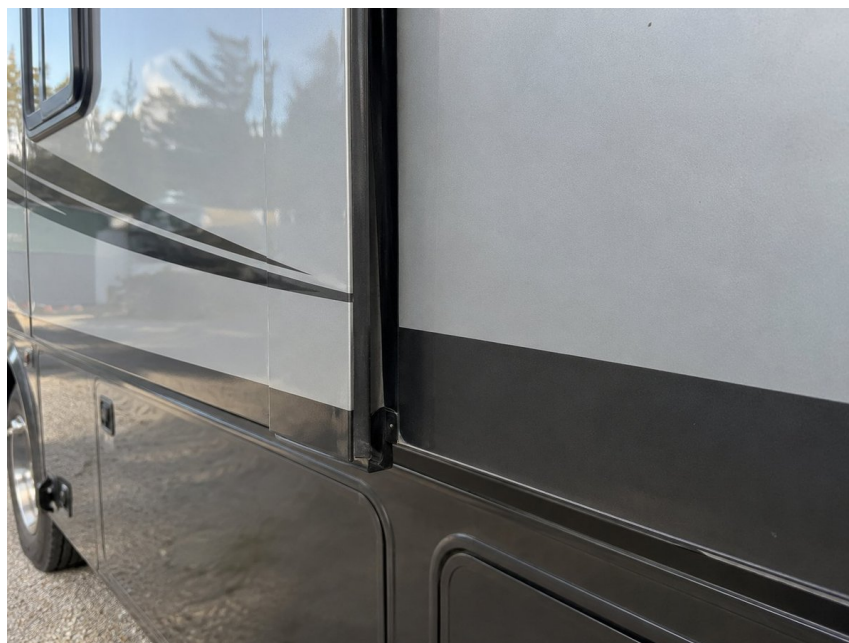
Illustration: Uneven gap at the living-room slideout edge.
