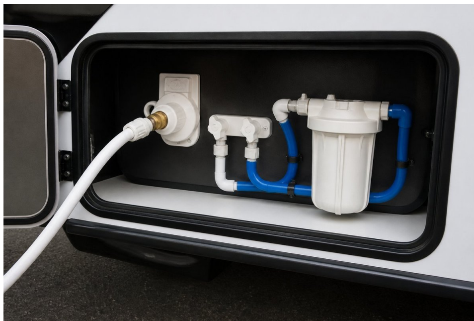
Illustration: City-water connection and filter compartment
